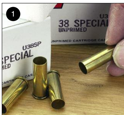
1. Using new brass, visually check all the cases for grit, packaging or brass chips before lubing, for steel dies, or running them into a carbide-sizing die.
