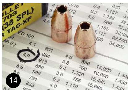
14. Consult a manual or other reliable loading data to ensure you are using the right powder and charge for the cartridge. In this example, we are using a Barnes 110-grain bullet and a starting load of 4.9 grains of Ramshot Zip pistol powder for a velocity of 918 feet per second (fps). Also, note the overall cartridge length is 1.435 inches with the bullet seated, which will allow it to function properly in any .38 Special revolver.
