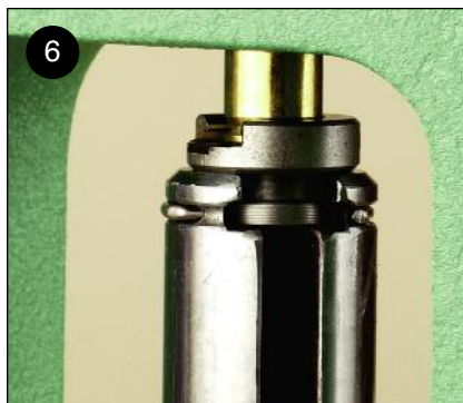
6. Raise the cartridge case into the die by running it up completely for full-length resizing. If it's a previously fired case, the primer will be expelled at this time. Clean the primer pocket with a few turns of the cleaning tool.
