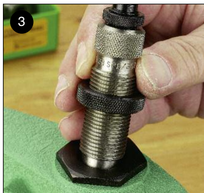
3. Insert the sizing (first of three) die into the press. Die sets are adjustable and allow the hand-loader to set the base of the die so it just touches the shellholder on the up or downstroke of the handle, depending on how the press is set up.
