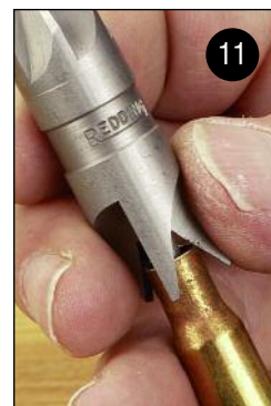
11. Turn the tool around and do the outside of the case mouth to remove burrs.
