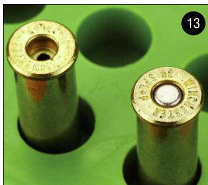
13. On the left is an unprimed case. On the right is the primed case flared and ready for a powder charge.
