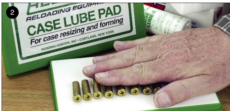
2. Lubricate all cases if you are using standard dies, but eliminate this step if carbide dies are employed. The latter are getting more popular for loading handgun ammunition, as they are cleaner and eliminate the need for cleaning all the cases after lubing.
