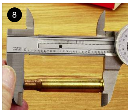
8. After sizing (new case out of the box) or resizing a case (after firing), check it for overall length.
