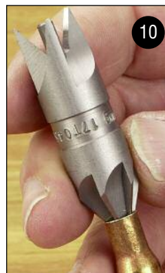
9. If your cases are over length, you have to trim them back to factory specifications. Like handguns, you can use either a trim die or a case trimmer, as illustrated here. A case trimmer utilizes a pilot in different diameters to fit most popular rifle cartridges.
