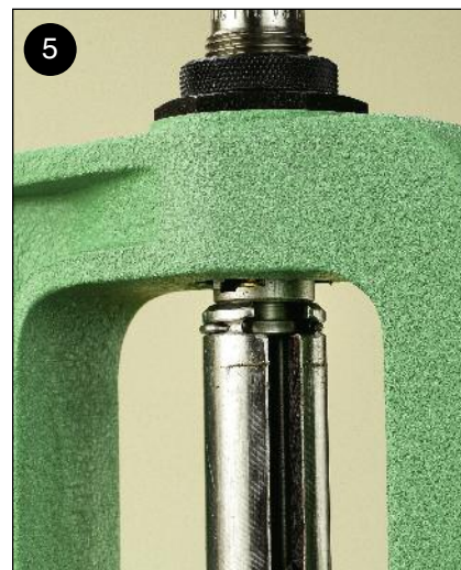
5. Run all the cases all the way up and into the sizing die. If a fired case is used, the primer will be expelled at this time also.
