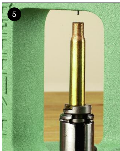
5. Slide a cartridge case into the shellholder, making sure it is touching the rear of the holder and enters the sizing die straightly.
