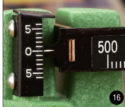
16. With all the various weights on the scale zeroed out, the far end of the scale must balance at zero.
