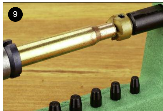
9. If your cases are over length, you have to trim them back to factory specifications. Like handguns, you can use either a trim die or a case trimmer, as illustrated here. A case trimmer utilizes a pilot in different diameters to fit most popular rifle cartridges.
