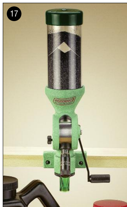
17. Now is the time to set up the powder measure on a rigid surface or use the screw clamps some companies offer.
