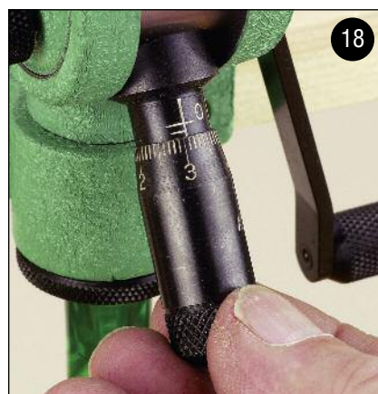
18. Adjust the powder measure to drop your load choice – from the loading manual. Adjust the measure until you get the exact weight, as confirmed on the powder scale.
