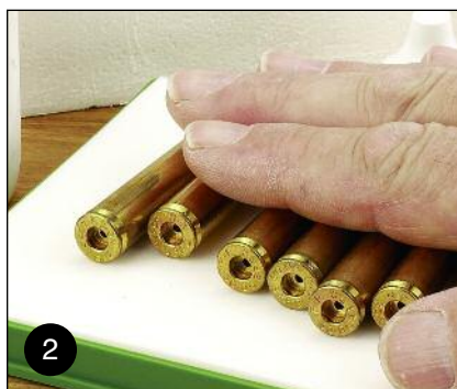
2. Lube all the cases sparingly before they go into the sizing die. Take a half-dozen or so, roll them on the lube pad, then one by one insert them into the sizing die.
