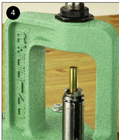
4. Insert the cartridge case (we are using the .38 Special throughout this sequence) in the shellholder that you installed on the press.
