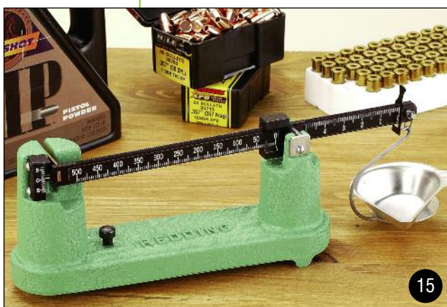
15. The next step is set up the scale and zero it. With faster-burning powders like Bullseye, attention to details is mandatory, as over-charging could result in damage to the firearm and the user.
